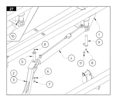
11 is fastened, attach self-locking nut 10 to screw 11 as show in figure, to prevent pin 9 to go out if screw 11 is loosened. Fasten cylinders 4 to fixed arms 2 & 3 (LH - RH) with pins 5, washers 6 and screws 7. Attach grease nipples 8 to pins 5.
