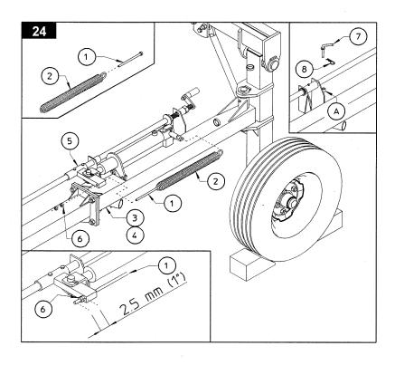
(LH - RH) and attachments 5 as shown, fastening the spring-bolt assembly in place with nuts 6. Pasten stay bolts 1 with nuts 6 so that they extend 25 mm (1") from attachment 5, as shown.
