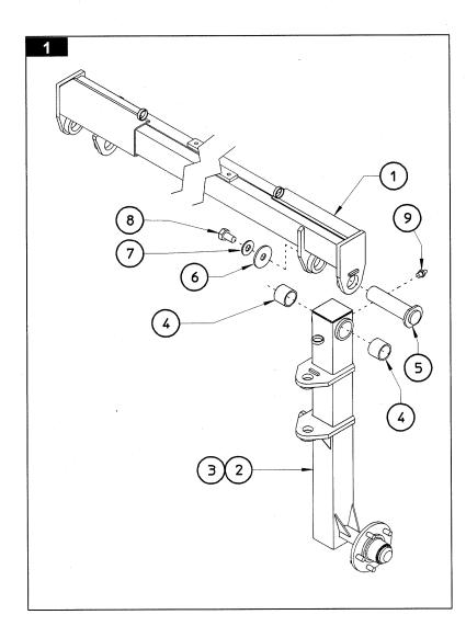
cross member assembly 1 using pins 5, washers 6 & 7 and screws 8. To identify parts 2 & 3 (LH - RH) see the next step.
