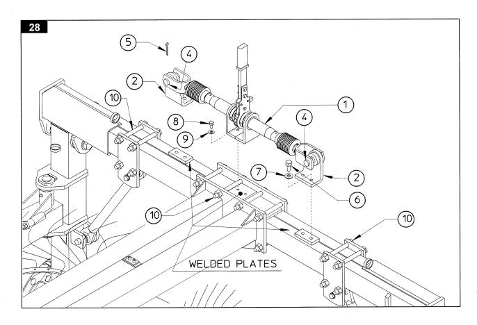
assy 1 to the machine with pins 4 and split pins 5, screws 8 and washers 9. Then tighen the screws 8 and 6.
