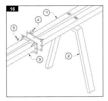
suitable capacity or support 2 (weight 110 kg, 245 lbs.). Attach drawbar section 3 (weight 65 kg, 145 lbs.) to drawbar section 1 using screws 4 and nuts 5.
