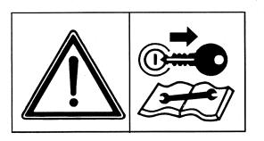
B) Before doing any maintenance or repair work, stop the machine at a suitable spot. Turn off the tractor motor, apply the brake, remove the key from the ignition and consult this manual.
