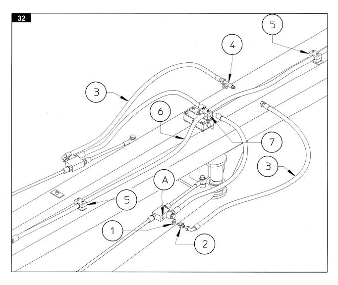
valve. Connect the curved end of hose 3 to nipple 2. Join hoses 3 to T connector 4 at the center of the machine.
