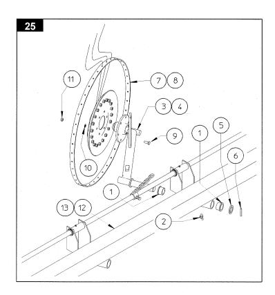
Attach rake wheel brackets 3 & 4 (LH - RH) to sections 12 & 13 (LH - RH) and fasten with washers 5 and spring pins 6. Mount rake wheels 7 & 8 (LH - RH) to rake wheel arms 3 & 4 (LH - RH) and fasten with screws 9, grower washers 10 and nuts 11. In this step, you will use:
