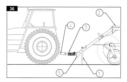
that drawbar 2 is parallel to the ground. Back the tractor up to the machine and look to see if hitch 3 is aligned with tractor hitch 4. If hitch 3 is much higher or lower than tractor hitch 4, it is necessary to change the position of hitch 3 by choosing the holes in plate 5 which give the best alignment. At this point connect hitch 3 to tractor hitch 4 using a suitable pin. Next turn the parking stand crank to retract the base of the stand.
