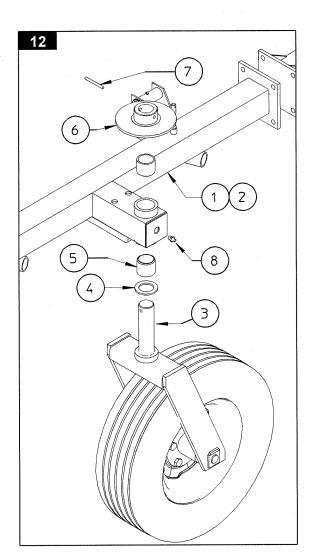
antifriction washer 4 on the pin of wheel assembly 3, and insert the wheel assembly pin in the correct holes in sections 1 & 2 (LH - RH) and secure it with the flanged bushing 6 and the spring pin 7. Attach grease nipples 8 to the correct holes of sections 1 & 2 (LH - RH).
