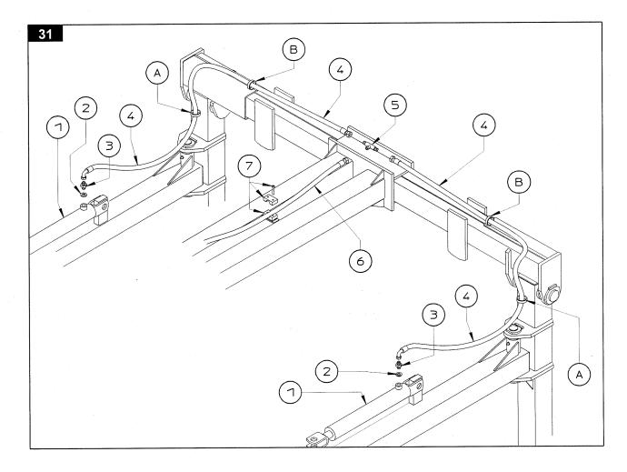
Pass hoses 4 through rings A & B and connect to T connector 5 at the center of the machine. Connect hose 6 to T connector 5 and secure in place with collars 7. NOTE: Hose 6 will also be in the next few steps.
