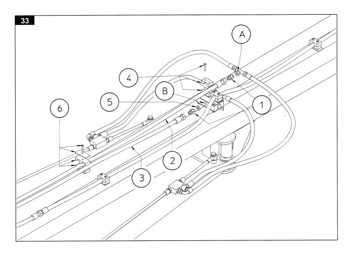
place with collars 4. Screw nipple 1 and washer 5 into hole B of the flow divider. Screw hose 3 onto nipple 1 and secure in place with hose collar 4. NOTE: Hoses 2 & 3 will also be in the next step.
