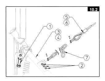
In order to increase and decrease interference between the side-delivery rake wheels, various positions can be selected to fasten the rake wheel holder supports (see point 7)
