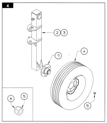
Item 5: 10 - nuts M 16 (5/8"), fine pitch and spherical cap.
