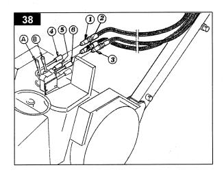
couplings 4-5-6. The movements of the machine are now controlled by operating levers A & B. Hoses 1 & 2, connected to couplings 4 & 5, control the cylinders for opening the machine. Hose 3, connected to coupling 6, controls the cylinders for lifting the rake wheels. It is recommended that all movements be repeated a few times to eliminate air from the system. The machine is now ready for operation.
