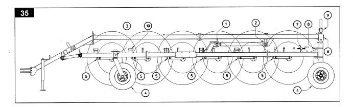
lubricate and check the movement of all parts. This diagram gives the maintenance program, to be carried out in its entirety the first time, and subsequently according to the schedule as shown.
